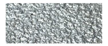
The guidelines shown below must be observed to insure that the galvanizing process does not damage SlipNOT® steel treated materials. SlipNOT® is not responsible for damage caused by third party operations such as galvanizing. Note: Damage to the SlipNOT® surface is caused from over exposure to pickling acids.
